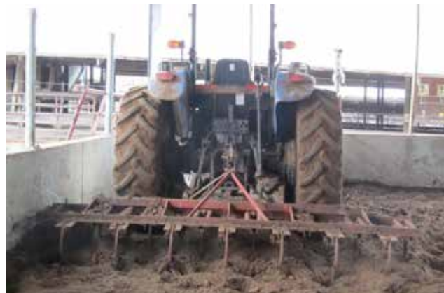
Figure 47. Sweeps or shovels may be added to tillage implement tines to provide more effective stirring. This is a cheap and effective addition to existing implements
