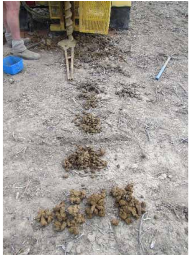
Figure 2. Layers of soil extracted from investigation using a drill rig
