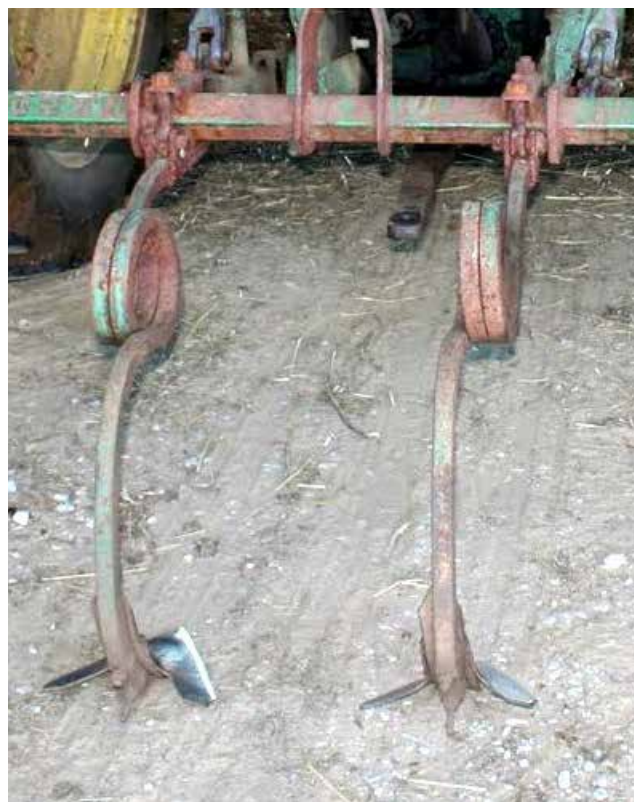
Figure 47. Sweeps or shovels may be added to tillage implement tines to provide more effective stirring. This is a cheap and effective addition to existing implements
