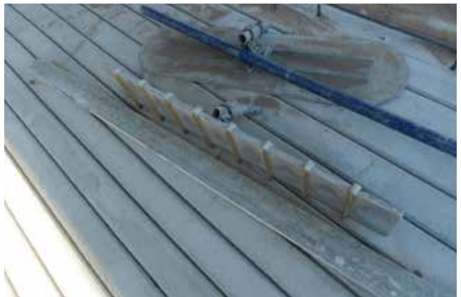
Figure 71. A typical float used to groove wet concrete
