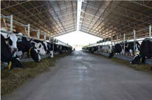
Figure 40. Eave overhangs can help minimise the amount of wind, precipitation, and sunlight entering the barn
