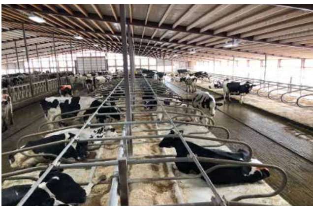
Figure 52. A three-row pen with a single row of stalls along the side wall
