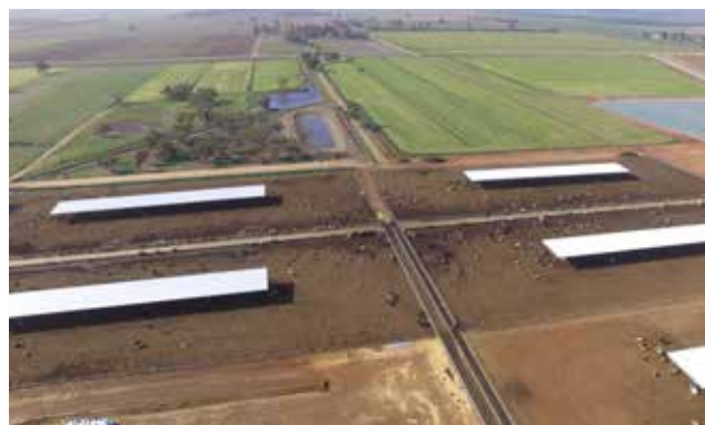
Figure 27. Aerial image of a well-designed dairy dry lot with north-south shade structures and central feeding table
