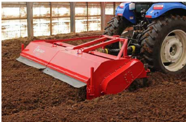
Figure 48. Roto-tillers may be used and are helpful to break up clumps of bedding material and maximize oxygen/air infiltration into the pack providing a uniform mix of material
